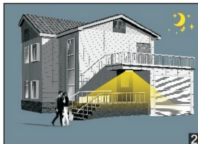
With insufficient daylight,even when motion detected.light ON.
